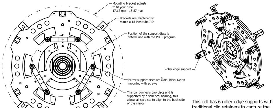
This cell has 6 roller edge supports with traditional clip retainers to capture the mirror and is suitable for all focal lengths. Mirror thickness of .8-2.0 in. 20-51mm
