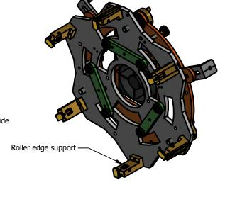
This cell has 6 roller edge supports with traditional clip retainers to capture the mirror and is suitable for all focal lengths. Mirror thickness of .8-2.0 in. 20-51mm
