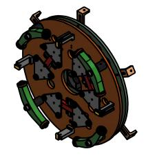
This cell has 4 whiffletree edge supports and traditional clip retainers to capture the mirror. It is suitable for mirror thickness of 1.0-2.0 in. 25-51mm and all focal lengths
