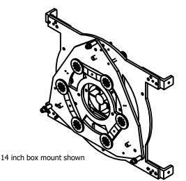
This cell uses silicone RTV to hold the mirror in place and is suitable for all focal lengths
