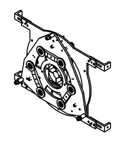
This cell uses silicone RTV to hold the mirror in place and is suitable for all focal lengths, and thickness of 1 - 1.95 inches.
