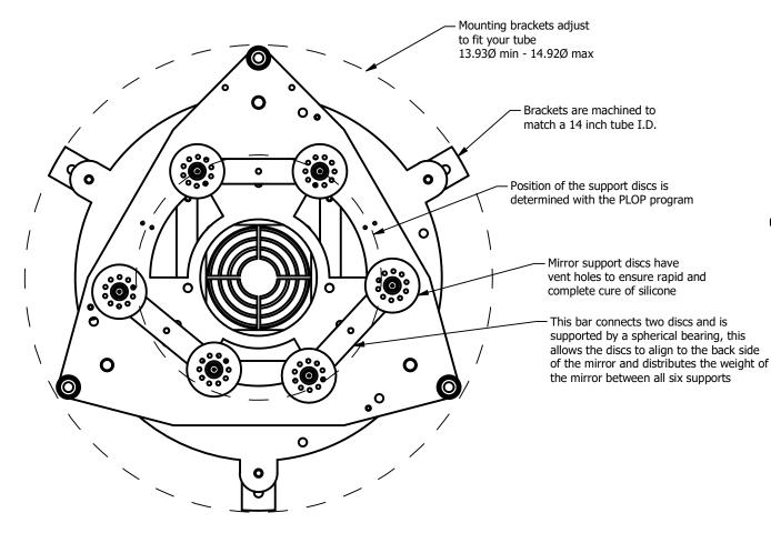
This cell uses silicone RTV to
