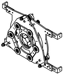
This cell uses silicone RTV to hold the mirror in place and is suitable for all focal lengths and thickness of .70 - 1.95 inches.
