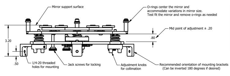
hold the mirror in place and is suitable for all focal lengths and thickness of .65 - 1.95 inches.
