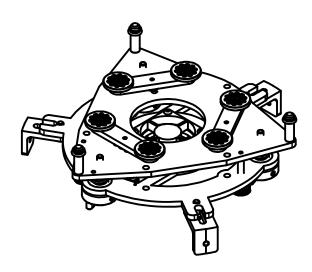
This cell uses silicone RTV to hold the mirror in place and is suitable for all focal lengths, and thickness of .70 - 1.95 inches.
